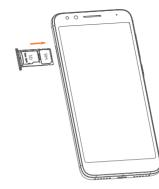
**Step 3.** Position the NANO SIM card or microSD card in the tray correctly, aligning the cutout tab, and gently snap into place. Be sure the edges are aligned.
