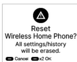
Press the Menu button twice to select OK action to proceed with the reset. After a factory reset, all settings will be restored to factory defaults, and call history data will be erased. To cancel the reset, after the above screen appears, press the Menu button once, or wait for 10 seconds.
