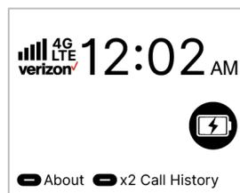
4. Check the signal strength indicator (
