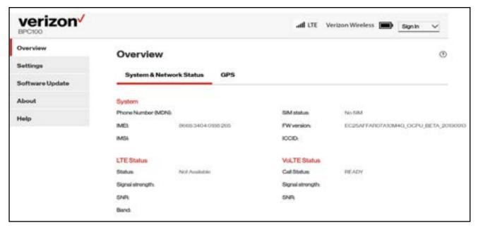
Select the **GPS** tab to display GPS coordinates of the current location of the BPC100. Latitude, longitude, altitude, and accuracy are shown as defined by GPS NMEA strings.
