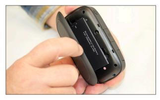
Insert your finger into the battery removal divot and lift the battery out of the battery compartment.
