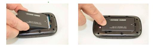
G Replace the cover by setting it on the Jetpack where the notches align, then press on the cover until it clicks into place and is flat across the entire bottom surface.
