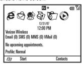
You can switch between the home screens by pressing and holding the home screen toggle key (A) on the keypad. (See page 2 for key location.)
