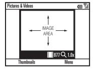
**Tip:** In either full screen or regular view, press the right soft key ( ) (Menu) to adjust picture settings, such as Mode, Brightness, Resolution, Zoom, White Balance, and Flash or switch to the video camera.
