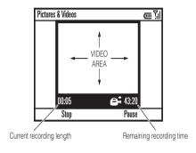
**Tip:** In the video viewfinder, press the right soft key () (Menu) to adjust video settings, such as Still, Brightness, Quality, and White Balance, or switch to Full Screen mode.
