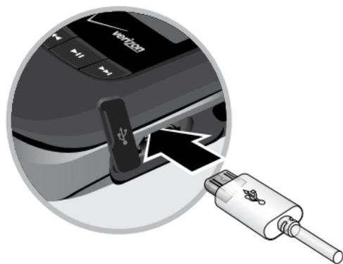
1. Open the side slot and plug the connector of the travel adapter jack into the jack on the side of the phone.
