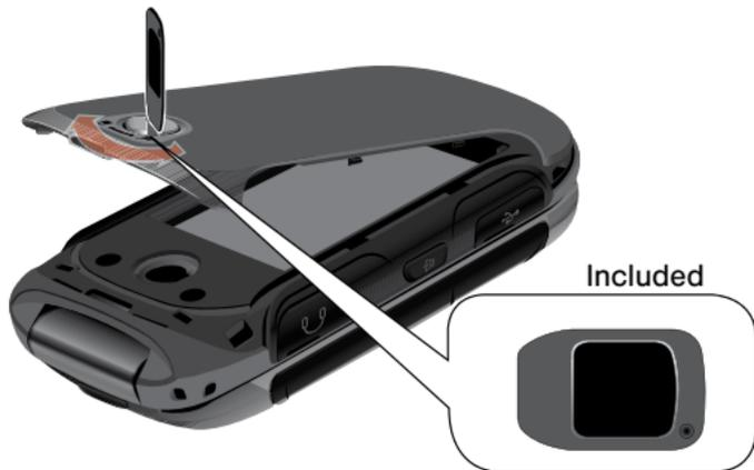
1. Use an object, such as a coin, and insert it in the slot on the back cover lock. Turn the lock counter-clockwise to open the battery cover. Lift the cover up and away from the phone.
