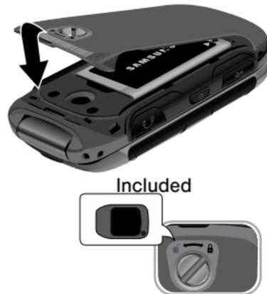
1. Place the cover back on the bottom of the handset then press down firmly.
