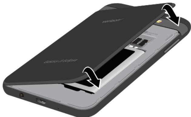
2. Press along the edge of the back cover until you have a secure seal.
