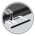
• Make sure that the card's gold contacts face down into the device and that the card is positioned as shown.
