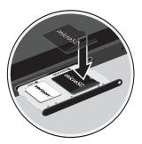
4. Slide the SIM card/Memory card tray back into the slot.
