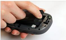
• Align the gold contacts on the new battery with the gold contacts on the Jetpack and gently slide the battery into place.
