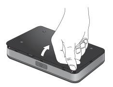
2. Align the gold contacts. Press down gently to secure the battery.
