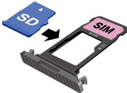
**NOTE:** If you need to reinstall your SIM card, remove the original SIM card from the tray and place your new SIM card into the tray with the gold contacts facing down as shown.
