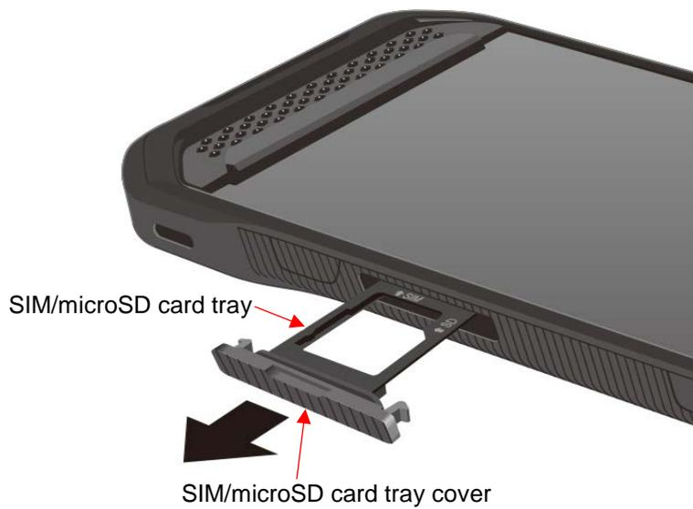
2. Put the tray onto a flat surface and place a microSD card into the tray. Ensure the gold contacts are facing down as shown.
