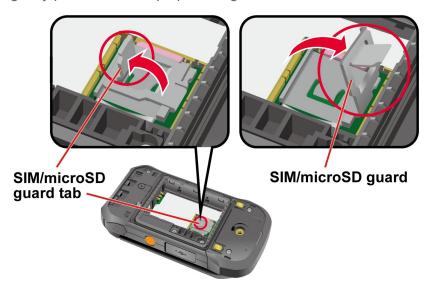
**Note**: Do not remove the SIM/microSD guard from the phone.
