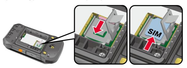
Note: Please be careful to not insert the SIM card into the SD card slot.
