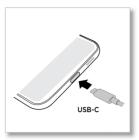
Charge your phone using a compatible Motorola charger (may be sold separately). Use of other chargers is not recommended. Insert the charging cable into the charging port (see **First look** for port location). Plug the other end into a power receptacle.
