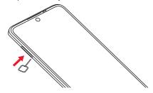
Step 2. Place the SIM card and/or microSD card into the tray, then slide the tray into the slot. It only fits one direction. Do not force into place. Keep the SIM tool in a safe place for future use.
