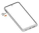
Step 2. Remove the NANO SIM card/microSD card tray.
