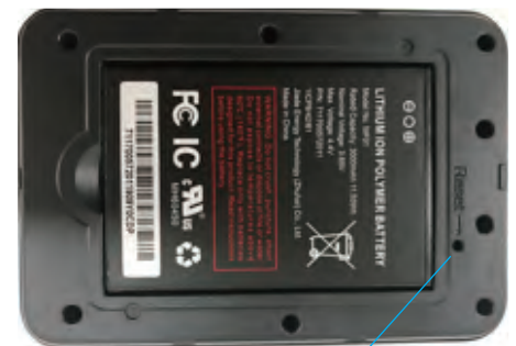
Factory Reset Pinhole
